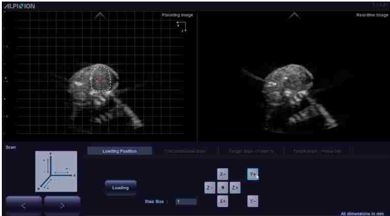
Figure 3.2 An example of user interface on aligning HIFU focus with the center of the pancreatic tumor. The mouse was positioned and tumor boundary was identified (white dashed line). A 3D positioner (along x, y, z axes) was used to move the animal holder, which was attached to positioning system, so that the HIFU focus (red cross) was aligned with the center of the tumor.
