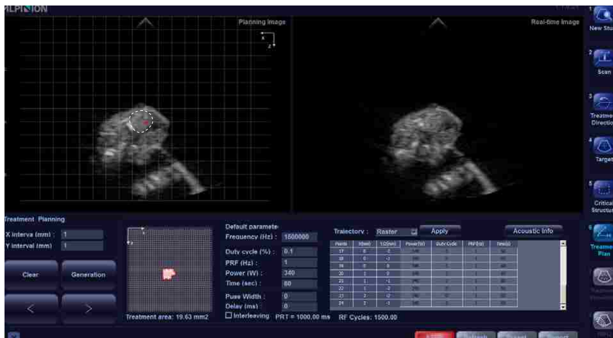
Figure 3.4 An example of user interface on treatment pattern generated across coronal plane of pancreatic tumor. After a separation distance is determined between two neighboring locations, a treatment grid was generated and parameters of duty cycle, pulse repetition frequency, electrical power and time duration for each spot were determined. The mouse was moved such that the treatment was performed in a raster pattern both laterally and vertically across the x, y plane.
